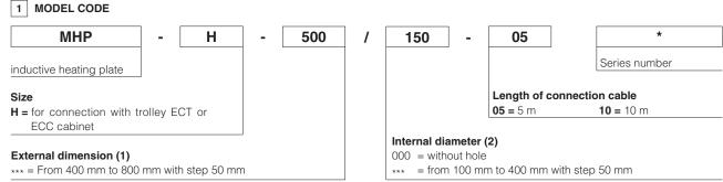
(1) The external dimension of the plate should be selected according to the mold surface; for example, in case of a rectangular mould, select the external dimension of the plate which is smaller than or equal to the length of the short side of the mould. See section 3 for available dimensions combinations.
