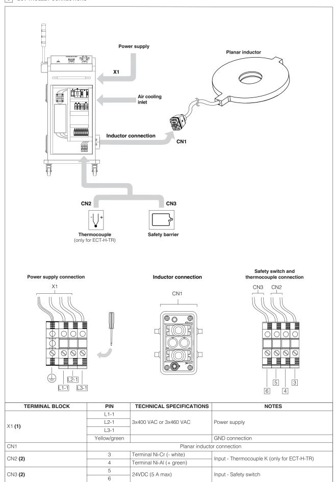
(1) Cable section: min.10 mm<sup>2</sup>; max.16 mm<sup>2</sup>; (2) Cable section max = 2,5 mm<sup>2</sup>
